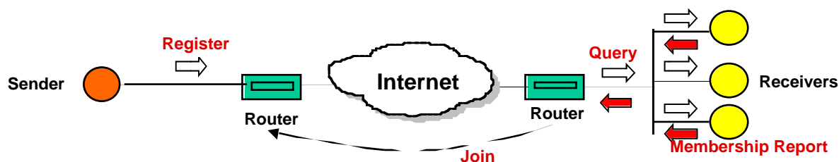
Figure 3: Receivers indicate which groups they wish to receive using IGMP, routers then identify the senders to this group and use a routing protocol to ask for the multicast packets.
